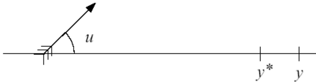
Figure 8. (a) An “archery” problem. (b) The parabolic relationship between distance traveled ( y ) and angle ( u ) for a projectile. For each value of y there are two corresponding values of u , symmetrically placed around 45 degrees.
