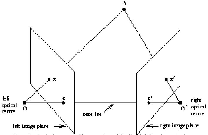
The **epipole**: is the *point* of intersection of the line joining the optical centres---the *baseline*---with the image plane. The epipole is the image in one camera of the optical centre of the other camera.
