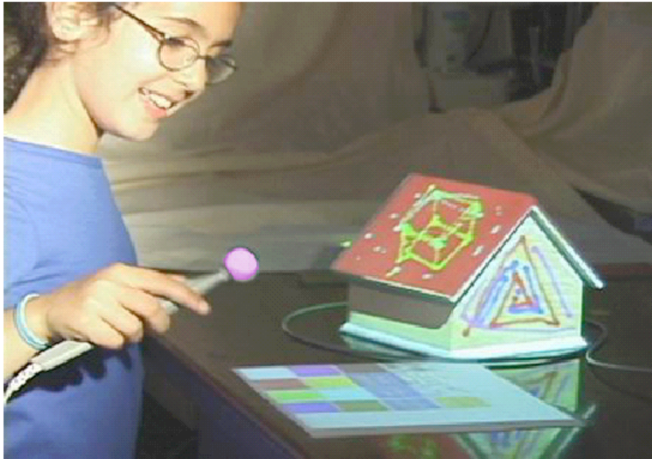
Figure 1. An enthusiastic young user (Miriam Mintzer Fuchs, age 9 years) demonstrates our easy to use system for 3D painting on movable objects. Note that the color palette on the table and the color on the spherical tip of the “paint brush” are projected.
