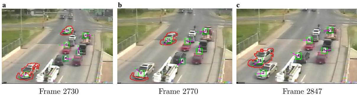
Fig. 8. Scene III: tracking in a crowded scene with stopped vehicles. The contours around the vehicles indicate the blobs detected. For vehicles not having the blob contour, the blob cue was missing.
