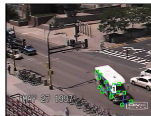
Fig. 1. A geometric template imposed on a target. The template consists of a spanning tree connecting the individual features on the target.
