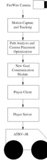
Fig. 8. Block diagram ATRV-JR camera system.
