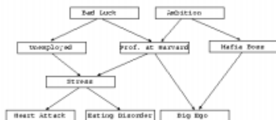
Figure 11 A Bayes Net is a directed graph with probabilities. The arrows derive links between nodes which directly influence each other. Imagine a gameshow where the players have to identify the professions of people but only by asking indirect questions. The jobs are “unemployed”, “Harvard professor” and “Mafia Boss”. The players are not allowed direct questions but they can ask about causal factors – e.g. “bad luck” or “ambition” – or about symptoms – “heart attack”, “eating disorder”, “big ego”.
