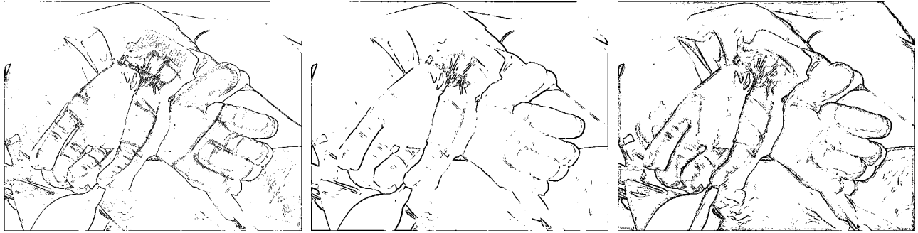
Figure 2.10 The edge estimated on the glove image by MAP with the filter at scale 0 (left), filter at scale 1 (centre), and filter with scales 0, 1, 2, 4 (right). Observe that the MAP estimates are significantly better than the ML estimates for this image. Also combining filters at multiple scales improves the performance.
