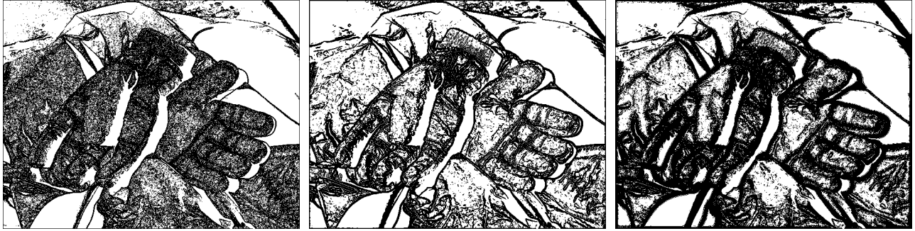
Figure 2.6 The edge estimated on the glove image by ML with the filter at scale 0 (left), filter at scale 1 (centre), and filter with scales 0, 1, 2, 4 (right). Observe that ML significantly overestimates the number of edges in this image.
