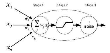
The generic neuron model abstracts the basic properties of the integrate and fire neuron, and makes provision for saturation as well.
