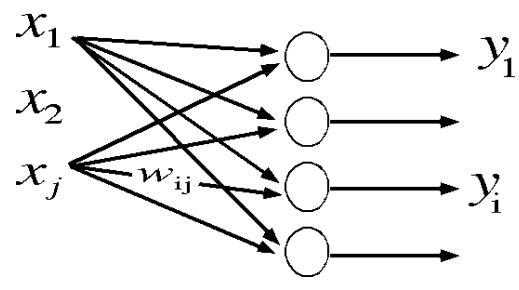
What if the input is applied to four neurons, each with a different set of weights? We can represent the weights by a "weight matrix", which is just a list of the four weight lists or vectors. Here is a 4x4 matrix W:
