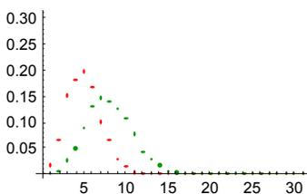
The horizontal axes represents a photon count, and the vertical axis represents the proportion of times that a particular count was measured. The histograms provide a quantitative representation of the variability. As the number of samples grows (i.e. test flashes in our case) , the histogram becomes a better and better approximation of a “true”, underlying Poisson distribution. Although we don’t prove it here, the Poisson distribution arises because of the independence of photon absorption.
