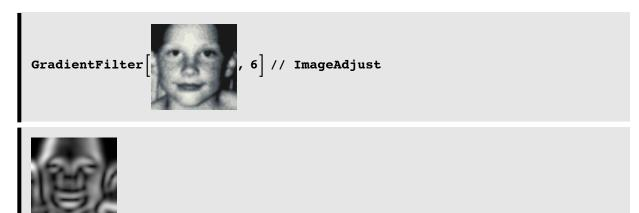
The  $\nabla^2 G$  operator in the previous lecture first convolves the image with a Gaussian blur kernel, and then takes the Laplacian  $\nabla^2$ .
