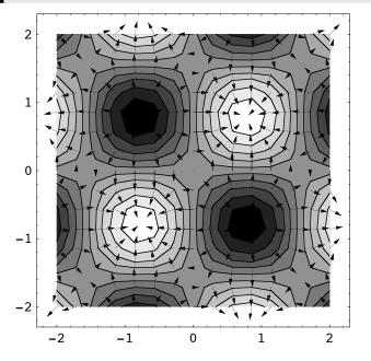
So each vector says which direction to take a step if you are climbing. And its length tells you how high a step you'll have to take. If you want to go *down* the landscape, just go in the direction given by the *negative* of the gradient, -gradZ[u,v]. The negative just turns the arrows around to put in the opposite direction. *Gradient descent* is what we will calculate below.
