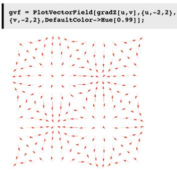
we see a set of vectors each of which always point towards the direction of local steepest ascent on the surface. **Note:** you can use the add-in function which will compute the gradient for you:
