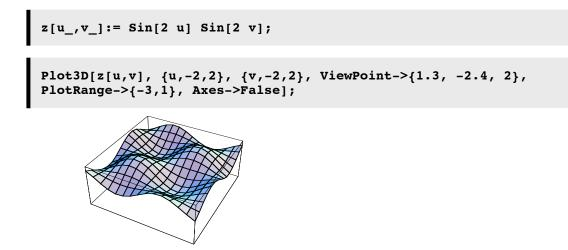
By eye, we can see roughly where the minima sit--there are two minima where z(u,v) = -1, i.e. at {Pi/4, -Pi/4} and {-Pi/4, Pi/4}. But imagine that z is a surface embedded in a much higher dimensional space. How then can we find the minimum when we can't just look at a plot and guess? Gradient descent is a method that will work in the 2D case, but can also be applied to much higher dimension like finding the optic flow (u's and v's) that minimze the above error function e.
