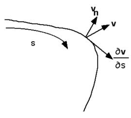
The smoothness is imposed by requiring that the rate of change of the contour velocity along the contour be small.
