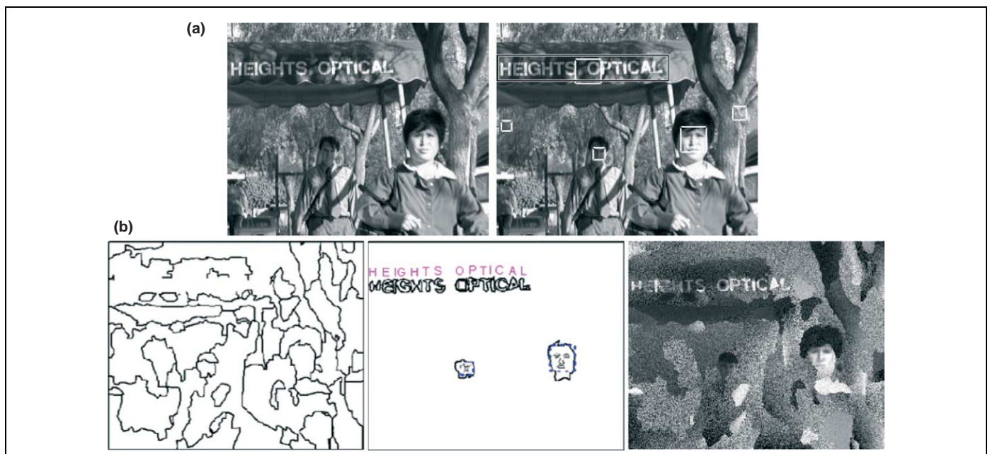
Figure 4. (a) Left: input image. Right: bottom-up proposals for text and faces are shown by boxes. A face is ‘hallucinated’ in a tree. (b) Left: overall segmentation. Centre: detection of letters and faces. Right: synthesised image.
