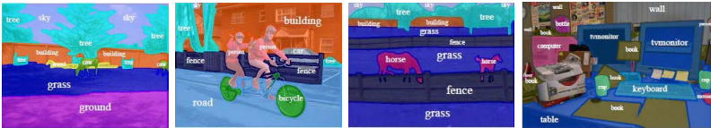
Fig. 24. Classifying local image patches. The image shows the groundtruth, see [119]. Certain classes – sky, grass, water – can be classified approximately from small image patches.
