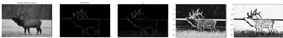
Fig. 22. The input image and its groundtruth edges (far left and left). The derivative dI/dx of the image in the x direction (center). The probabilities of the local filter responses P(\mathbf{f}(I(x))|y = 1) (right) and P(\mathbf{f}(I(x))|y = -1) (far right) have their biggest responses on the boundaries and off the boundaries respectively, hence the log-likelihood ratio \log \frac{P(\mathbf{f}(I(x))|y=1)}{P(\mathbf{f}(I(x))|y=-1)} gives evidence for the presence of edges.
